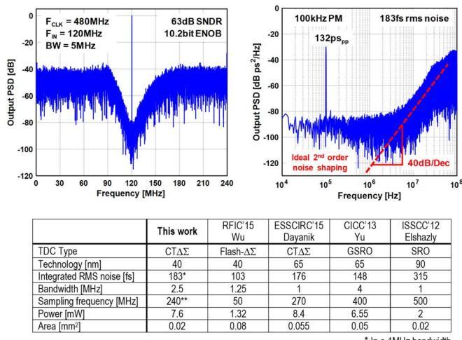
Figure 15.3.4: Measured BPDSTM and BPDSTDC output power spectra (top) and comparison of noise-shaping TDCs (bottom).
