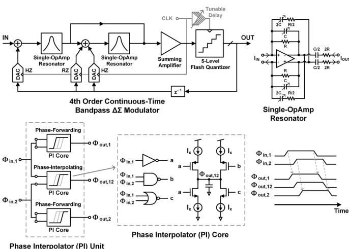
Figure 15.3.3: Bandpass  $\Delta\Sigma$  modulator with resonator circuit (top) and PI unit cell with PI core circuit (bottom).
