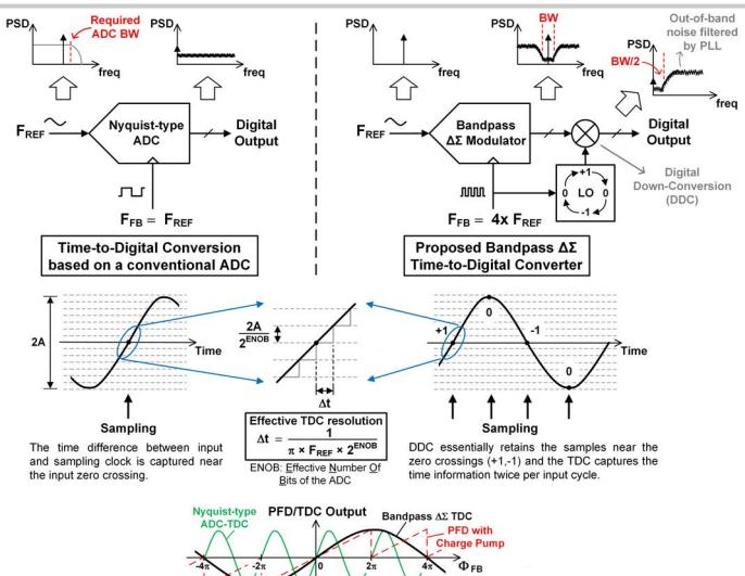
Figure 15.3.1: Nyquist-type ADC-TDC vs. Bandpass  $\Delta\Sigma$  TDC (top and center) and phase transfer curves (bottom).
