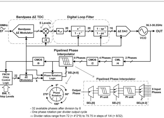
Figure 15.3.2: Fractional-N chirp synthesizer PLL (top) and pipelined phase interpolator (bottom right).
