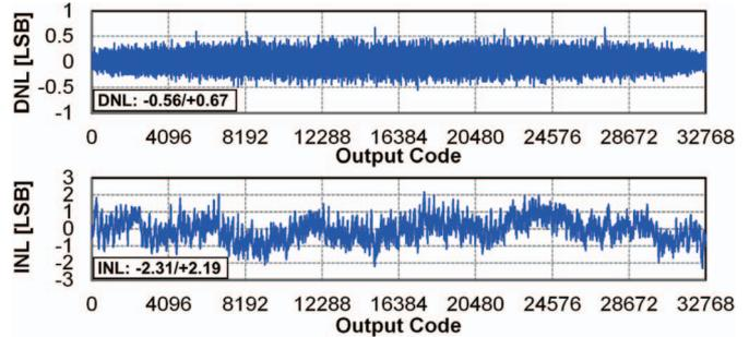
Fig. 6: Measured Linearity.
