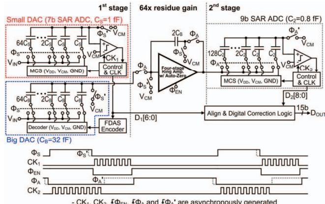
Fig. 4: Block diagram and timing of the ADC (Actual implementation is fully differential).
