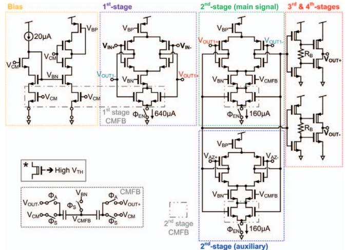
Fig. 1: Four-stage fully differential ring amplifier and biasing.
