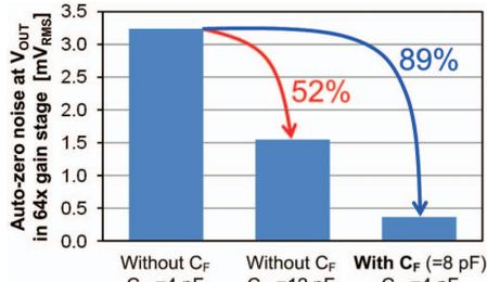
Fig. 3: Auto-zero noise filtering transient noise simulation.
