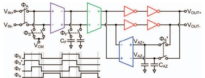
Fig. 2: Simplified four-stage ring amplifier in auto-zero configuration and timing diagram.
