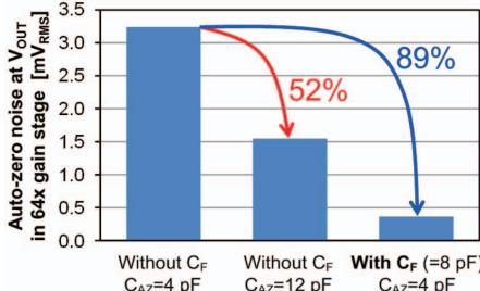
Fig. 3: Auto-zero noise filtering transient noise simulation.
