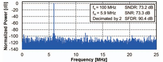
Fig. 7: Measured Spectrum (2<sup>20</sup> point FFT).
