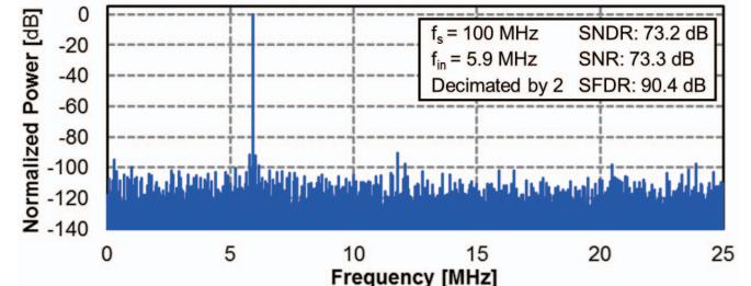
Fig. 7: Measured Spectrum (2<sup>20</sup> point FFT).
