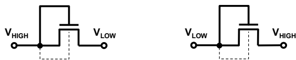
Figure 4 – A well bias with a fixed connection to either the source or drain can lead to the well being set to too high a voltage leading to reverse leakage.
