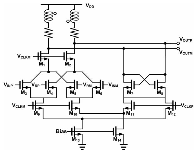
Fig. 1. Comparator core.
