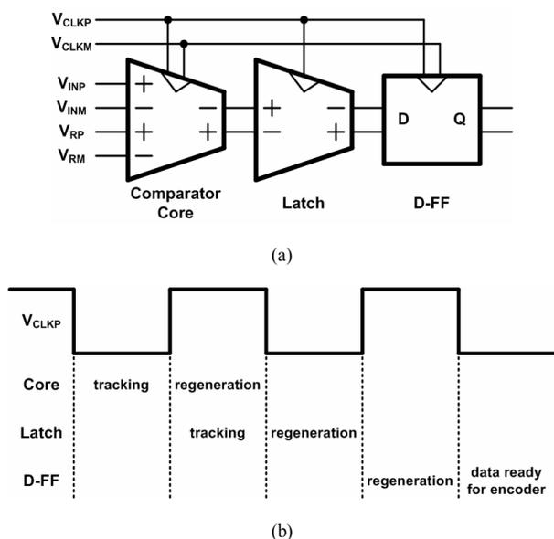
Fig. 3. Comparator unit with timing diagram. (a) Comparator unit. (b) Timing diagram.
