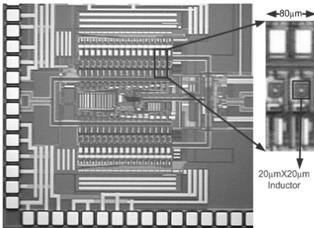
Fig. 8. ADC micrograph, with a magnified view of two comparators.
