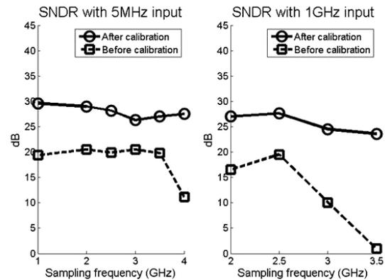
Fig. 10. SNDR with 5MHz and 1GHz input frequencies.
