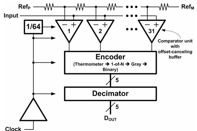
Fig. 7. ADC architecture. (Offset correction logic not shown for simplicity)
