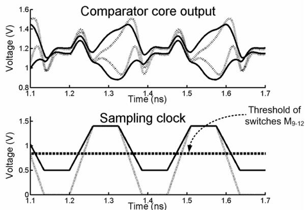
Fig. 2. Comparator core output waveforms with different clock amplitude (0.9 V and 1.4 V).
