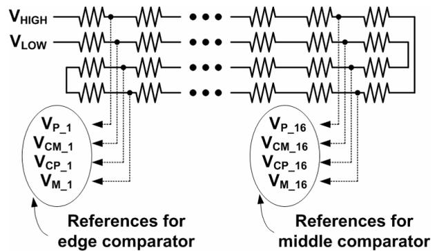
Fig. 6. Resistor ladder implementation.
